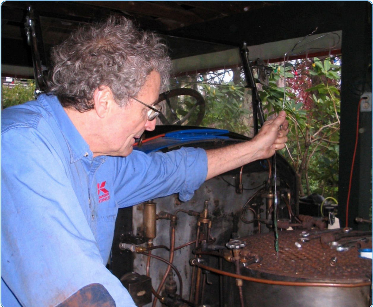
Ian cleaning the bonier tubes before swaging
